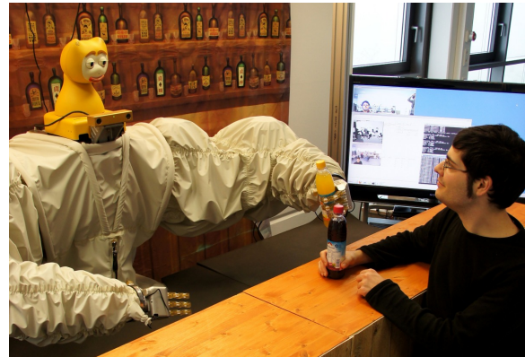
Figure 1: The robot bartender of the JAMES project uses head pose estimation to infer the state of interaction of human customers in a multi-party bar scenario.
