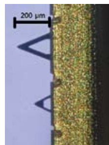
Fig. 2: Photograph of two force sensors used for force spectroscopy experiments.
