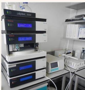
The **preparative HPLC** has many applications in research and in the industry as well. It is used for the isolation, the purification of relevant molecules, and to study the stability of drugs. With this device, it is also possible to perform quality control analysis as it is the case in the pharmaceutical industry.
